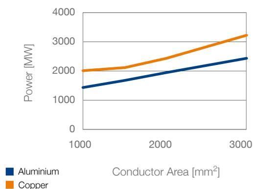
Figure 2. Transmitted power as a function of conductor area and metal for a cable pair. The copper (3000 mm<sup>2</sup>) and aluminum (2000 mm<sup>2</sup>) 640 kV cables are shown in right.
